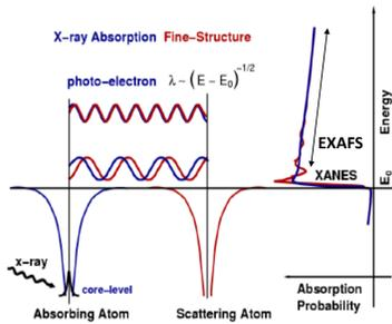
X-ray Absorption Spectroscopy (XANES/EXAFS) probes local atomic and electronic structure as well as lattice dynamics.
