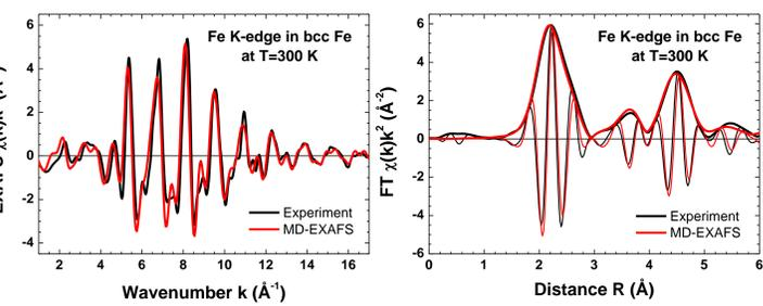
Validation of Embedded Atom Model (EAM) force field model for Fe from M.W. Finnis and J.E. Sinclair, Phil. Mag. A 50 (1984) 45.
