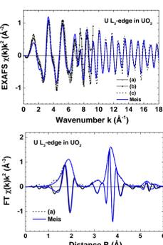
Comparison of the experimental and calculated U L<sub>3</sub>-edge EXAFS  $\chi(k)k^2$  and their Fourier transforms (FTs) for UO<sub>2</sub> at T = 300 K. The experimental EXAFS signals correspond to (a) UO<sub>2</sub>, (b) irradiated Cr-doped UO<sub>2</sub> and (c) non-irradiated undoped UO<sub>2</sub>. The configuration-averaged EXAFS signal was calculated by the MD-EXAFS method at T = 300 K using the core-shell potential of Meis et al.
