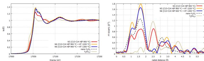
Y K-edge XANES (on the left) and FT-EXAFS (on the right) for ODS samples HIP 900°C (red), after heat treatment 1220°C (orange), 1300°C (blue), and nano-Y<sub>2</sub>O<sub>3</sub> (black dash), Y<sub>2</sub>Fe<sub>17</sub> (olive dotted) reference samples.
