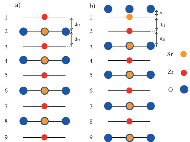
Fig. 2. Sketch of the side views of slab geometries used to study SrZrO<sub>3</sub> (111) surfaces. (a) Non-stoichiometric nine-layer slab with Zr-terminated surfaces. (b) Non-stoichiometric nine-layer slab with SrO<sub>3</sub>-terminated surfaces with definitions of surface rumpling *s* and the near-surface interplanar separations  $\Delta d_{12}$  and  $\Delta d_{23}$ .
