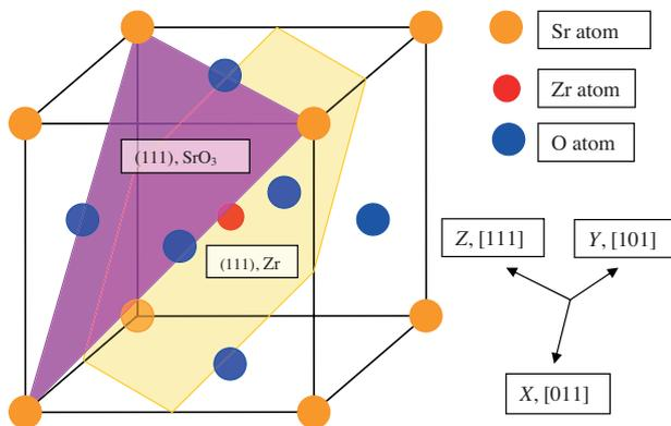
Fig. 1. Sketch of the cubic SrZrO<sub>3</sub> perovskite structure showing two possible (111) surface terminations: SrO<sub>3</sub> and Zr.
