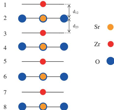
Fig. 3. Sketch of the stoichiometric eight-layer slab with Zr and SrO<sub>3</sub>-terminated (111) surfaces with definitions of the near-surface interplanar separations  $\Delta d_{12}$  and  $\Delta d_{23}$ .
