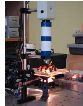
Helmholtz coils for creation time dependent magnetic field
