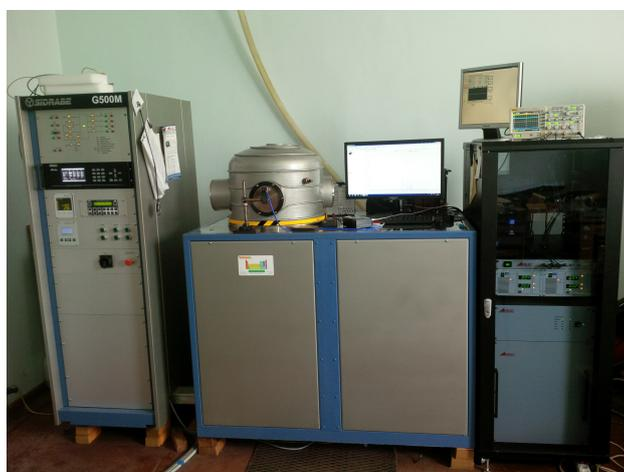
Figure 4.1.1. Vacuum sputter system Sidrabe G500M.
