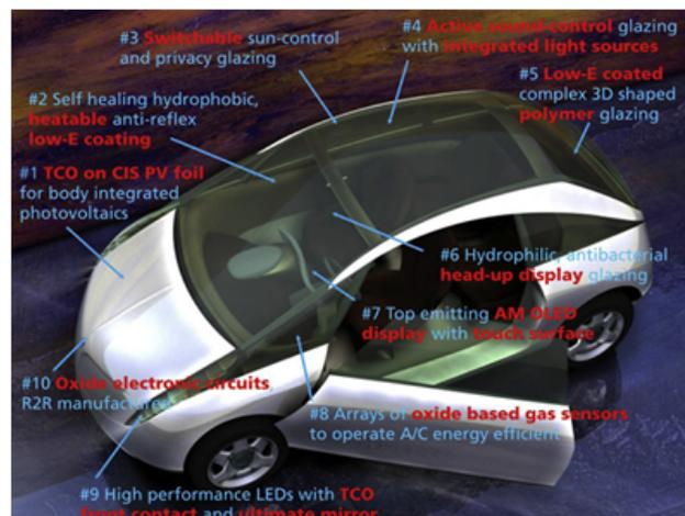
**Figure 1.1.1.** A vehicle equipped with the potential technologies which require transparent conducting materials [18].
