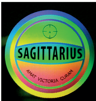
Pic. 3.6.1. Photo of surface relief-phase grating. Recorded in KRJ-8 film without etching post-treatment. Recording duration – 15h, diameter – 13.5mm.
