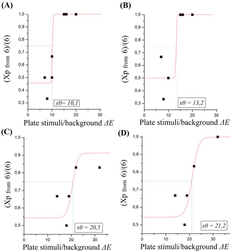
**Figure 13.** Color discrimination thresholds of participant KS (acquired with KAMS2). Graphs (A) and (B) show threshold values acquired with reddish plates in first and fifth (last) measurements respectively. Graphs (C) and (D) show threshold values acquired with greenish plates in first and fifth (last) measurements respectively.
