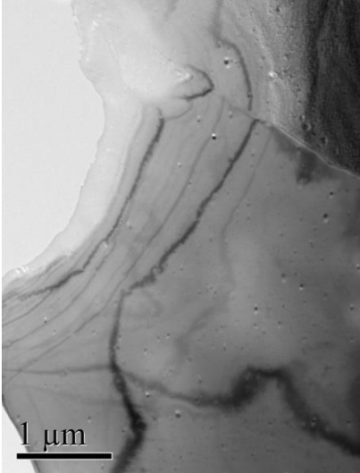
Figure 1.1. Transmission electron microscope (TEM) image of the ferritic steel.
