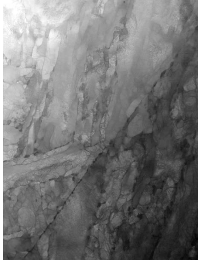
Figure 1.2. TEM image of the martensitic steel ( 12.1\ \mu\text{m} ).
