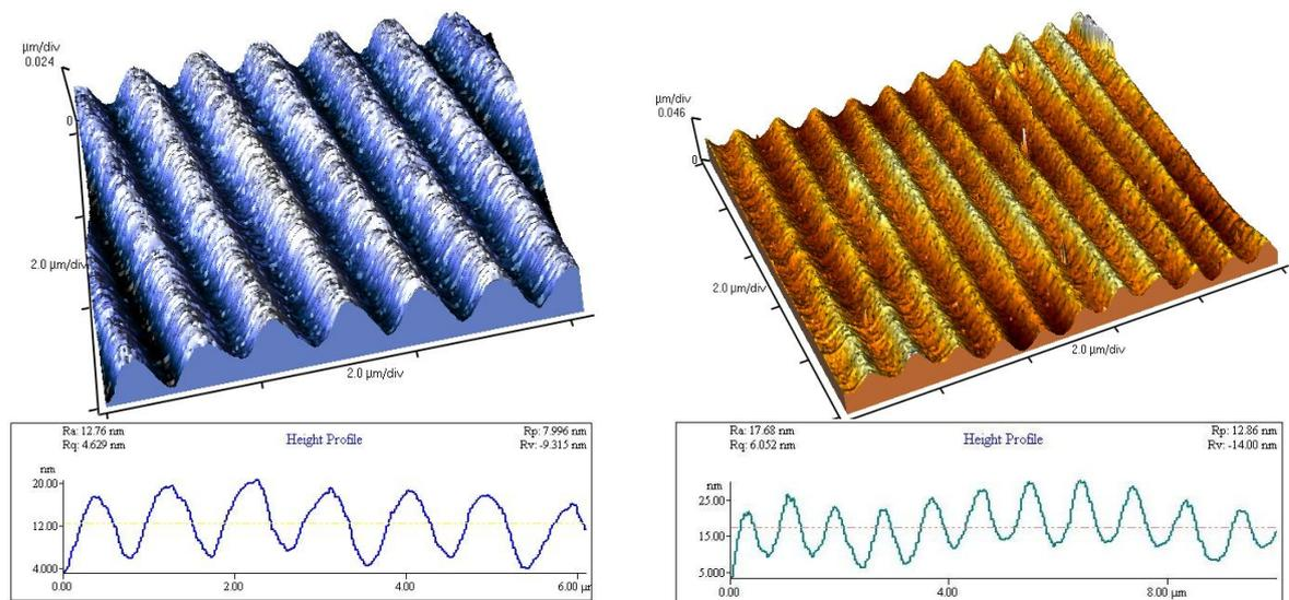
Figure 8. AFM images of surface relief and profiles of holographic gratings recorded by laser 532 nm in composites 40%  $\text{As}_2\text{S}_3$  - 60% Disperbyk161 (blue) and 5% DR-1 - 35%  $\text{As}_2\text{S}_3$  - 60% Disperbyk161 (yellow), film with thickness  $\sim 5 \mu\text{m}$ .
