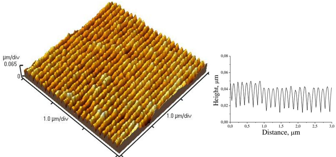
Figure 5. AFM image and profile of grating with period 130 nm, recording by immersion method.
