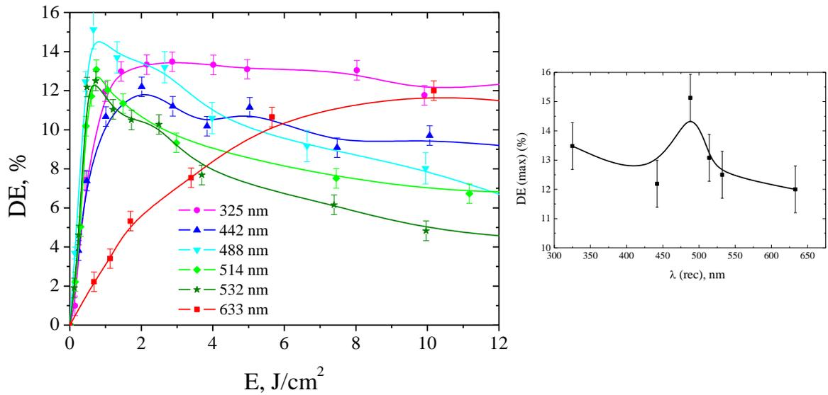
Figure 2. Dependence of reflection DE of grating in photoresist  $As_{40}S_{15}Se_{45}$  on recording exposure after dissolution for different recording wavelength. Reading laser 441,6 nm. Additional graph shows the dependence of maximum reflection DE on recording light wavelength.
