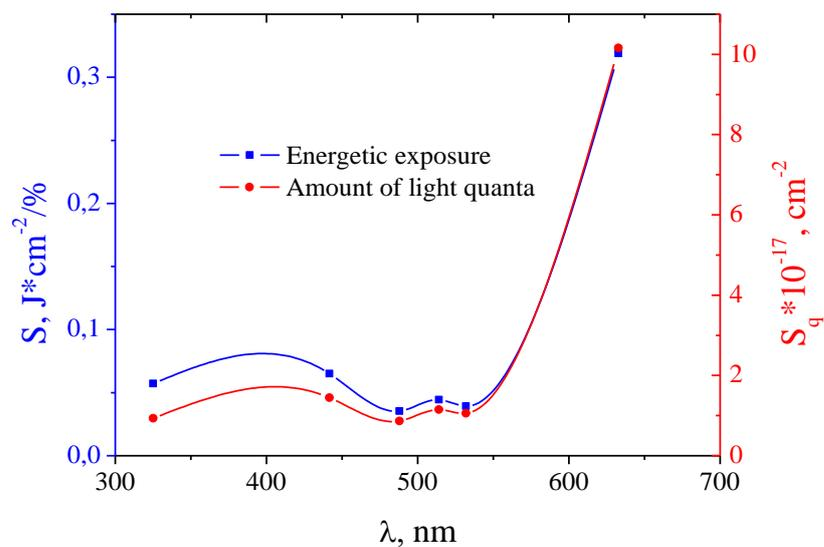
Figure 3. Spectral sensitivity of photoresist  $As_{40}S_{15}Se_{45}$ .
