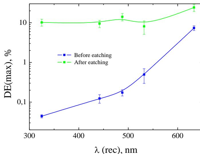
Figure 1. Dependence of maximums of transmission DE of gratings in photoresist  $\text{As}_{40}\text{S}_{15}\text{Se}_{45}$  on recording light wavelength before and after etching. Reading laser 670 nm at Bragg angle.
