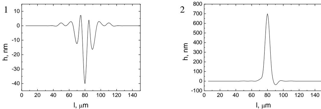
Figure 7. Character of relief of composition 40%  $\text{As}_2\text{S}_3$  + 60% Disperbyk 161 (1) and composition 5% DR1 + 35%  $\text{As}_2\text{S}_3$  + 60% Disperbyk 161 (2) after laser irradiation of composites through cylindric lens by laser beam 532 nm.
