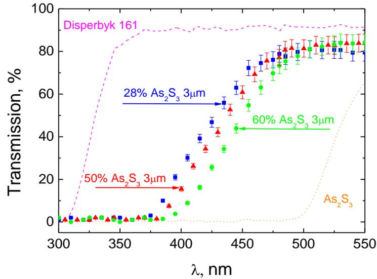
Figure 6. Transmission spectra of  $\text{As}_2\text{S}_3$ /Disperbyk 161 composite films dependence on  $\text{As}_2\text{S}_3$  concentration.
