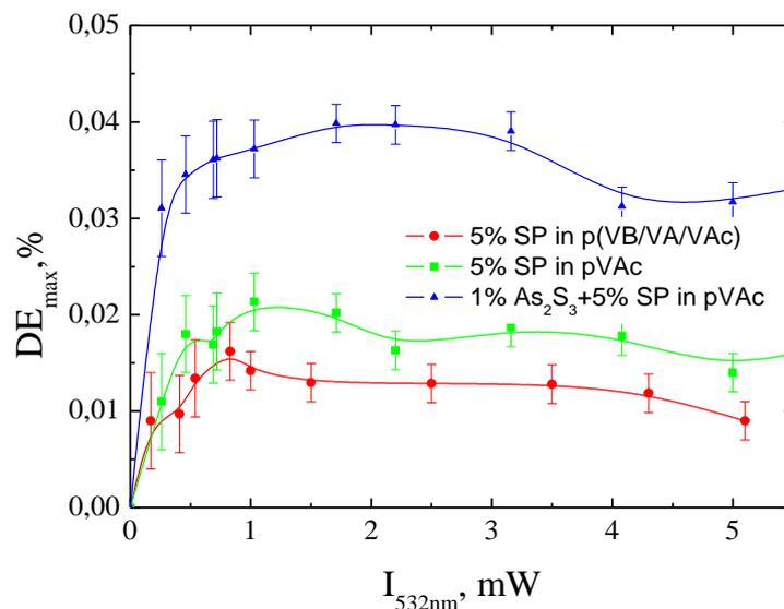
Figure 8. Dependence of transmission DE maximums on the recording beam intensity (recording and reading lasers 532 nm).
