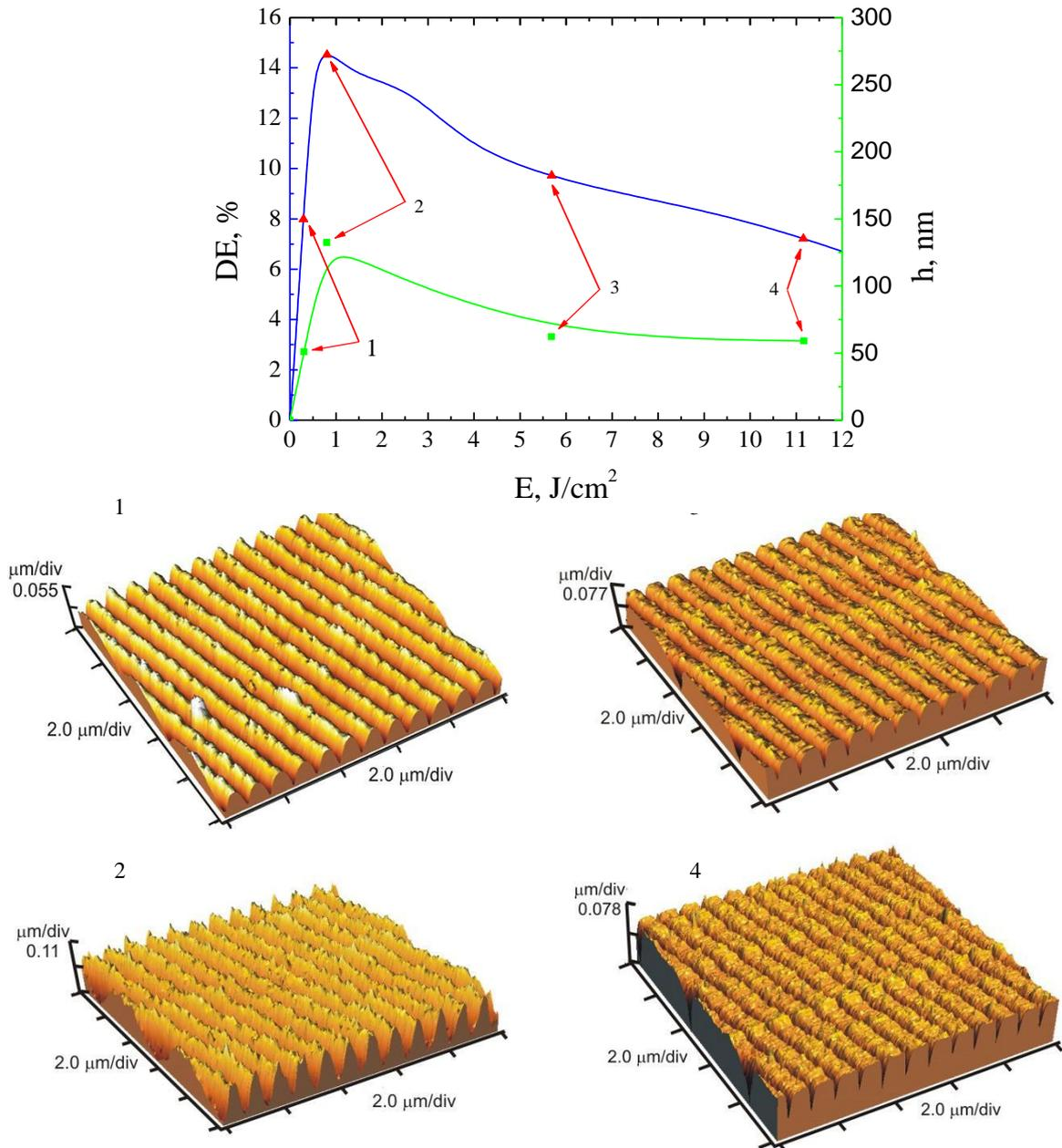
Figure 4. The dependence of DE of gratings in photoresist  $As_{40}S_{15}Se_{45}$  after etching, recorded by laser 488 nm (blue) and the dependence of relief height of gratings (green) on recording exposure and AFM images of gratings.
