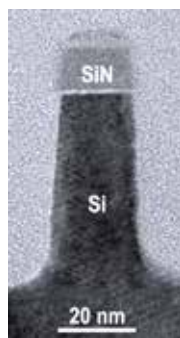
Silicon fins and trenches etched from PPA resist.
