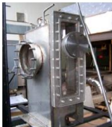
Mock-up of the jets entrance region. Three d=3mm liquid metal jets.
