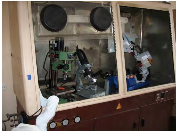
Figure 4.1.1. Workplace for mechanical treatment of carbon-based tiles
