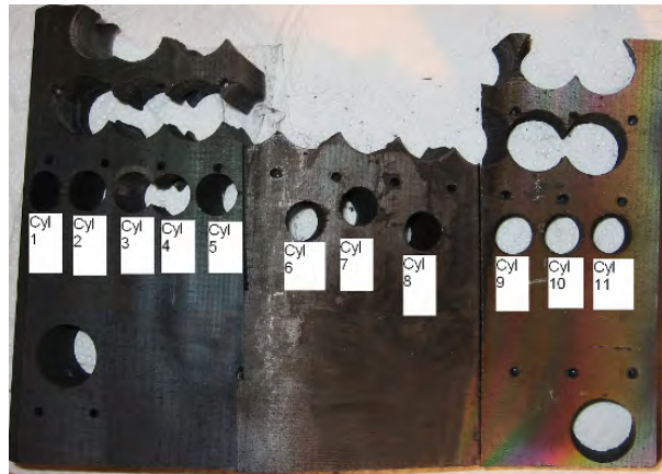
Figure 4.1.2. Core drilling positions of tile 14 BWG4B
