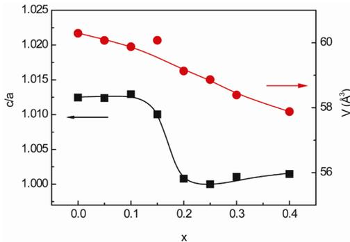
**Figure 3.12. Concentration dependences of unit cell volume and tetragonality for  $0.4\text{NBT}-(0.4-x)\text{ST}-0.2\text{PT}-x\text{CaTiO}_3$  solid solutions**
