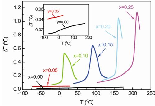
**Figure 3.8. ECE temperature change  $\Delta T$  as a function of temperature at  $E = 20$  kV/cm for 0.4NBT-(0.6-x)ST-xPT compositions with various PT concentrations  $x$**
