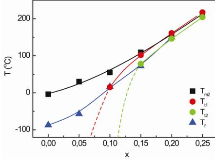
Figure 3.3. Phase diagram of 0.4NBT-(0.6-x)ST-xPT system of solid solutions: concentration dependence of phase transition temperature  $T_t$  on heating ( $T_{t1}$ ) and on cooling ( $T_{t2}$ ) and dielectric permittivity maximum temperature  $T_m$  on cooling ( $T_{m2}$ ) (at 1 kHz). At  $x = 0.10$  temperature  $T_{t1}$  is observed only for previously poled sample
