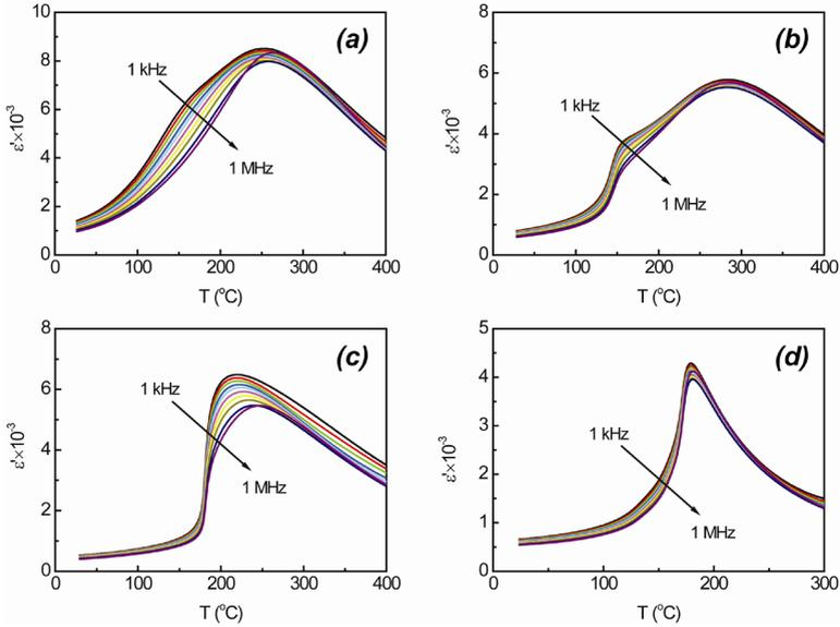
**Figure 3.14. Temperature-frequency dependences of dielectric permittivity, obtained on cooling, for (1-x)NBT-xBT compositions with BT concentrations a)  $x = 0.1$ , b)  $x = 0.2$ , c)  $x = 0.4$ , d)  $x = 0.9$**
