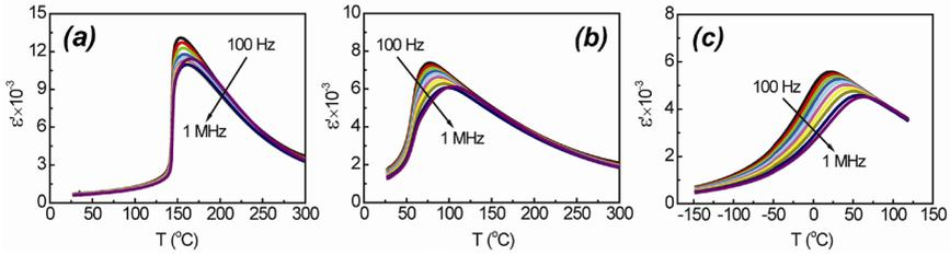
**Figure 3.11. Temperature dependences of dielectric permittivity at several fixed frequencies for  $(1-x)(0.4\text{NBT}-0.4\text{ST}-0.2\text{PT})-x\text{NN}$  solid solutions with NN concentrations  $x = 0.00$  (a),  $x = 0.04$  (b) and  $x = 0.10$  (c) (cooling curves)**
