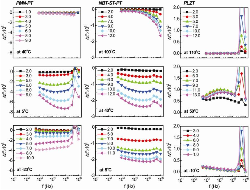
**Figure 3.6.** Difference between  $\varepsilon''$ , measured at different values of bias field  $E_{\pm} \neq 0$ , and  $\varepsilon''$ , measured at  $E_{\pm} = 0$ , as a function of frequency for compositions 0.92PMN-0.08PT, 0.4NBT-0.5ST-0.1PT and PLZT 9,25/65/35 at three different temperatures: above  $T_m$ , in the region of  $T_m$  and below  $T_m$  (values of electric field in the labels are given in kV/cm)
