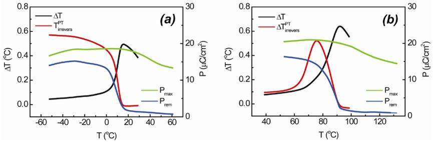
**Figure 3.10. Reversible  $\Delta T$  and irreversible  $\Delta T_{\text{irrevers}}^{\text{PPT}}$  temperature changes (measured at the first applied electric field for thermally depoled sample, corrected for the hysteresis heat), as well as maximal  $P_{\text{max}}$  (at 20 kV/cm) and remnant  $P_{\text{rem}}$  polarizations as functions of temperature for compositions 0.4NBT-0.5ST-0.1PT (a) and 0.4NBT-0.45ST-0.15PT (b)**
