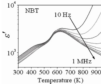
Figure 1.1. Temperature dependences of the real part of dielectric permittivity at different frequencies [3]
