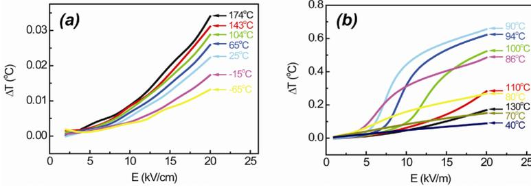
**Figure 3.9. ECE temperature change  $\Delta T$  as a function of electric field  $\Delta T(E)$  at different temperatures for compositions 0.4NBT-0.6ST (a) and 0.4NBT-0.45ST-0.15PT (b) (measurements are done for electric field change from 0 to different values)**
