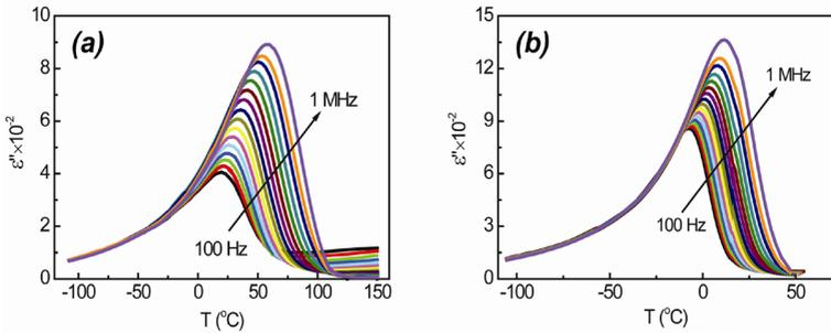
Figure 3.4.  $\varepsilon''(T, \omega)$  cooling curves for compositions a) 0.4NBT-0.5ST-0.1PT and b) 0.9PMN-0.1PT
