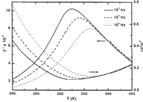
**Figure 1.3. Temperature and frequency dependences of the real part of dielectric permittivity  $\epsilon'(T,f)$  [19]**
