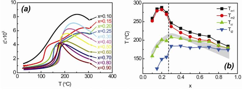
**Figure 3.15. a) Temperature dependences of dielectric permittivity for (1-x)NBT-xBT with various BT concentrations (cooling curves at 1 kHz); b)  $\epsilon'(T,f)$  maximum and phase transition temperatures  $T_m$  ( $T_{m1}$ ,  $T_{m2}$ ) and  $T_f$  ( $T_{f1}$ ,  $T_{f2}$ ) as functions of concentration, obtained at 1 kHz, for (1-x)NBT-xBT (the phase coexistence region, determined from x-ray diffraction heating measurements, is highlighted)**
