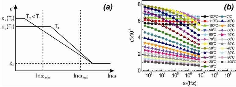
Figure 3.5. a) schematical representation of  $\epsilon'(\omega)$ , which illustrates the main features of dielectric dispersion; b)  $\epsilon'(\omega)$  for composition 0.4NBT-0.5ST-0.1PT
