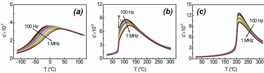
**Figure 3.1. Temperature dependences of dielectric permittivity  $\epsilon'$  at several fixed frequencies for 0.4NBT-(0.6-x)ST-xPT solid solutions at PT concentrations  $x = 0.05$  (a),  $x = 0.15$  (b),  $x = 0.25$  (c) (cooling curves)**
