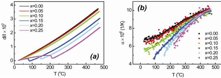
Figure 3.7. Temperature dependences of thermal expansion (a) and thermal expansion coefficient (b) for NBT-ST-PT compositions with various PT concentrations  $x$
