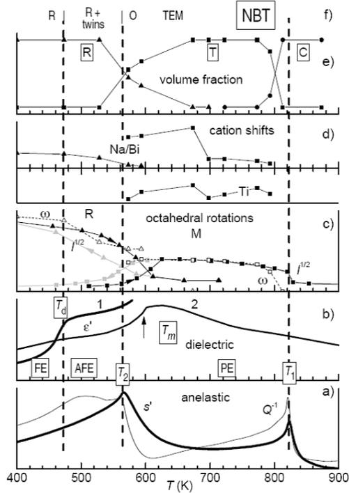
**Figure 1.2. Anomalies of different properties in NBT as a function of temperature: a) elastic properties; b) dielectric properties; c) octahedral rotations, obtained from neutron diffraction; d) cation shifts, obtained from neutron diffraction; e) volume fraction obtained from neutron scattering [12]**
