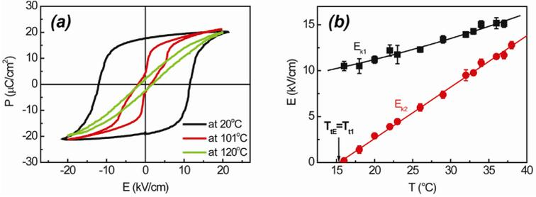
**Figure 3.2. a) Polarization hysteresis loops ( $P(E)$ ) for composition 0.4NBT-0.45ST-0.15PT at several temperatures; b) temperature dependences of critical electric fields  $E_{k1}$  and  $E_{k2}$  for composition 0.4NBT-0.45ST-0.10PT**
